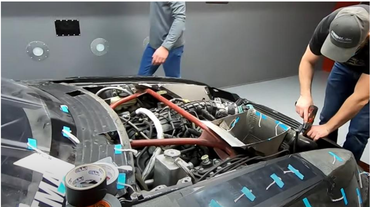
Rad Exit Ducting (back of radiator connected to hood openings via ducting)
