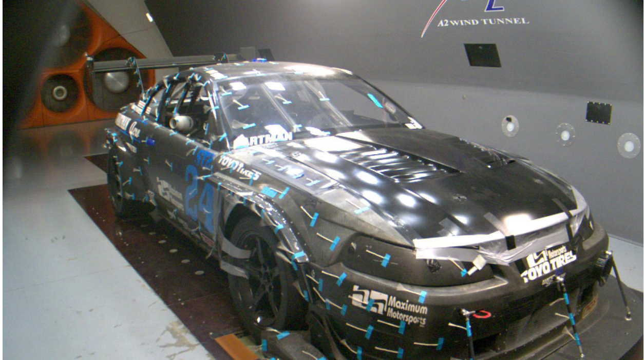
Carbon Fiber Extractor Hood (no radiator exit ducting, back of rad open to engine bay)
