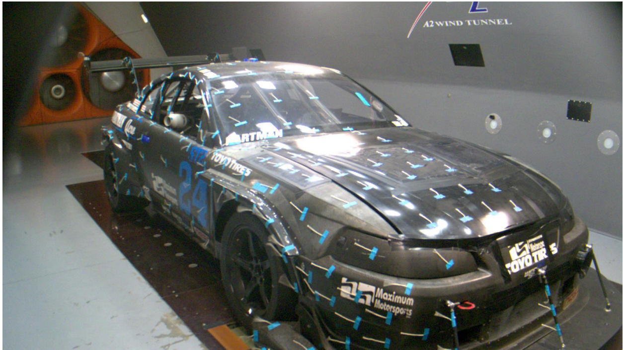
Baseline - Stock OEM Hood (no vents, no radiator exit ducting, back of rad open to engine bay)
