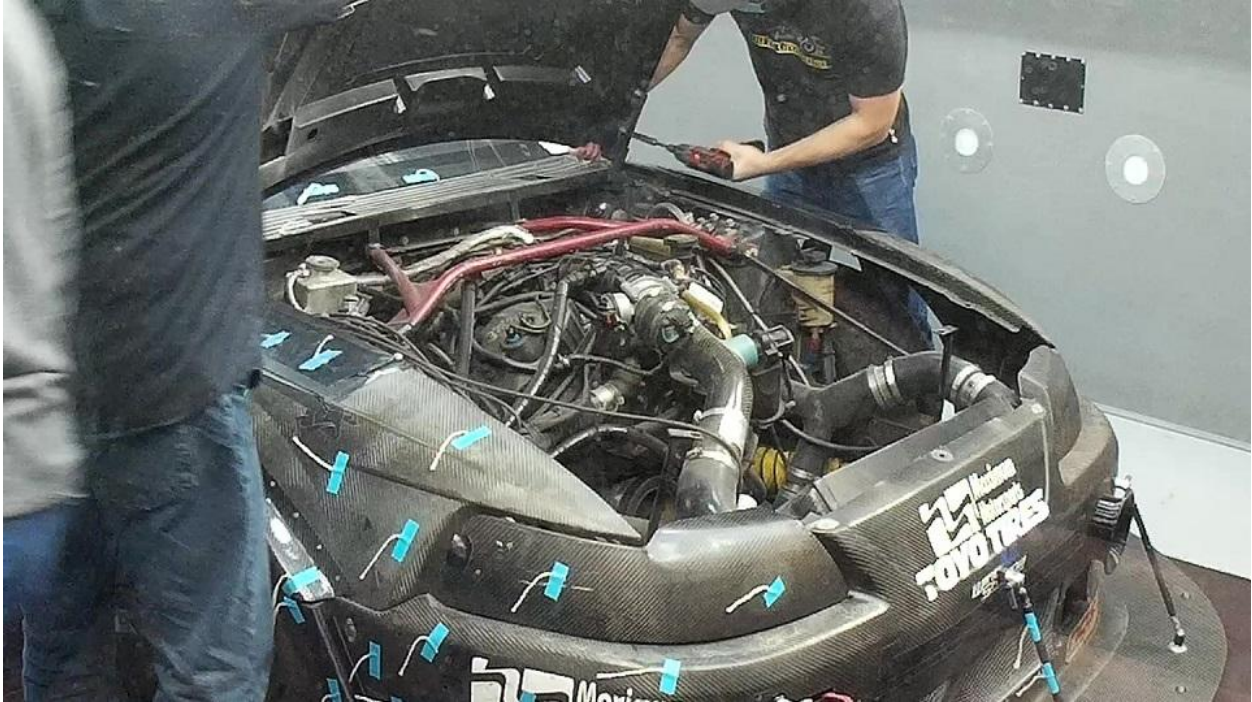
No rad exit ducting for OEM hood, Race Louvers and CF extractor hood tests (back of radiator open to engine bay)
