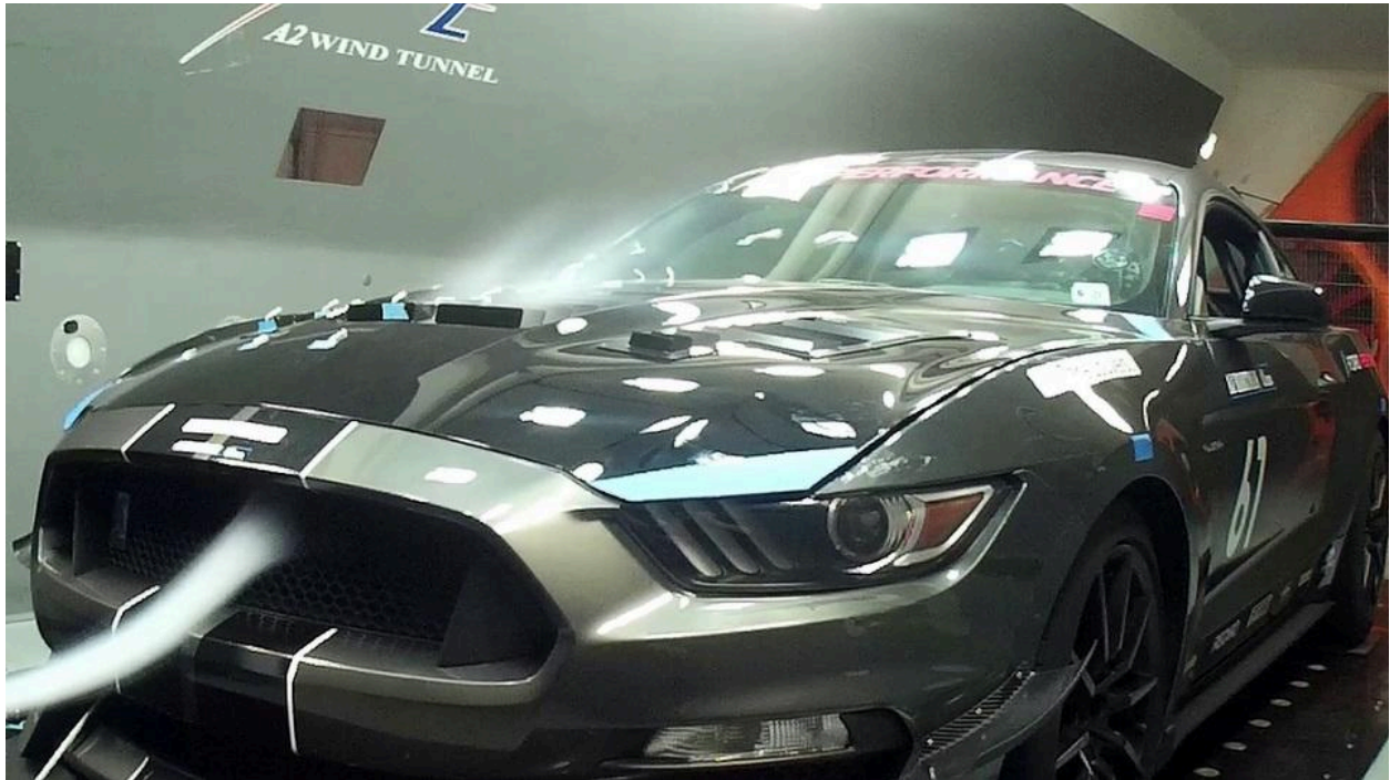
Fig 3 - Smoke Visualization Of Airflow Path
