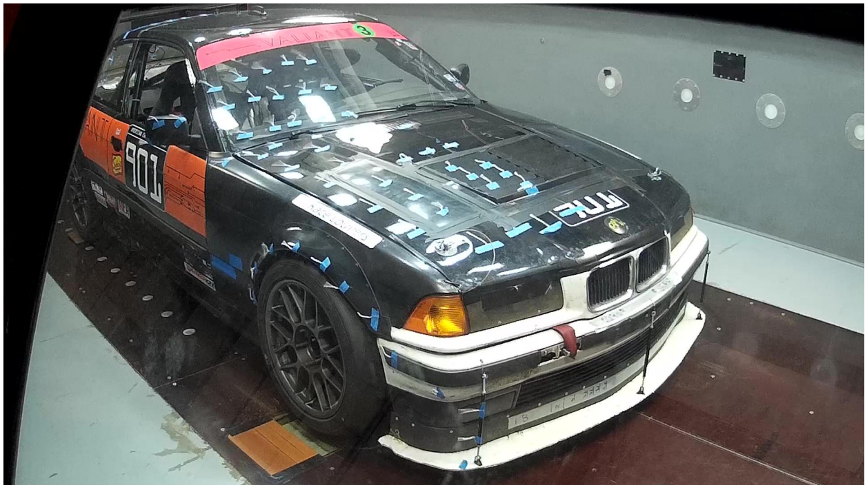
Recessed louvers with angled gurney flap 3/4" overall height
