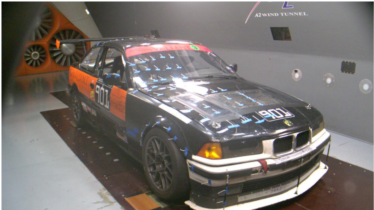
Baseline No Vents (holes sealed shut)
