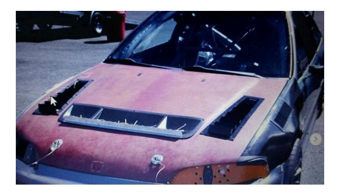
Customer: Rory A. Location: Washington Vehicle: Honda Civic Event type: Budget endurance racing Previous setup: GT500 center vent Extractor setup: Race Louvers RX trim side pair 235 sqin with GT500 center vent Temperature reductions: 235F to 210F coolant temp reduction
