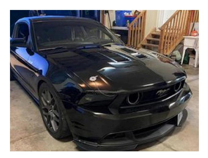
Customer: Ahmed K. Location: Texas Vehicle: 2012 Mustang GT Event type: Daily Driver Previous setup: No vents Extractor setup: Race Louvers RS street trim center hood louver pair, 310sqin total. Temperature reductions: 15F degree reduction in cruise temps.
