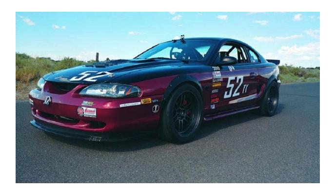
Customer: Sean T. Location: Nevada Vehicle: Cobra Mustang Event type: Road course racing Previous setup: No vents Extractor setup: Single center RT track trim 280 sqin Temperature reductions: 235F to 210F coolant temp reduction
