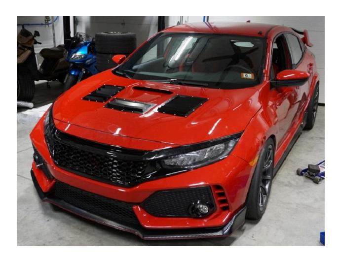
Customer: Don K. Location: New Hampshire Vehicle: 2018 Honda Civic Type R Event type: SCCA Time Trials Previous setup: No vents Extractor setup: Race Louvers RT center and side kits Temperature reductions: Now can run full 30 minute sessions in 90F heat where previously it would overheat after 3 laps.
