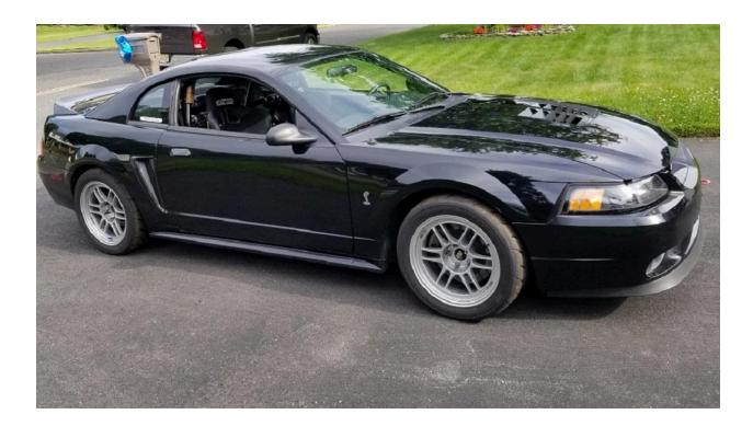
Customer: Peter F. Location: New Jersey Vehicle: Cobra Mustang Event type: High performance driving events Previous setup: No vents Extractor setup: Race Louvers single center recessed trim 240 sqin Temperature reductions: 230F to 210F coolant temp reduction
