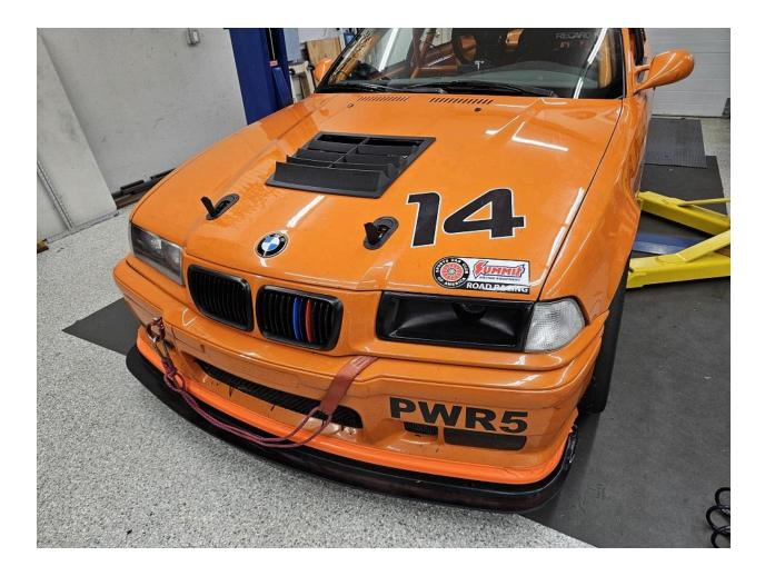
Customer: Marshall L. Location: USA Vehicle: BMW E36 Event type: Wheel to wheel racing Previous setup: No hood vents Extractor setup: Race Louvers CF Extreme center hood vent. Temperature reductions: 220+F to 200F coolant temp reduction
