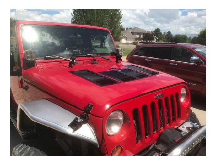
Customer: Chuck B. Location: Colorado Vehicle: 2008 Wrangler with LS swap Event type: Towing, high elevation Previous setup: No vents Extractor setup: Race Louvers RS street trim center hood louver and side hood louvers, 550sqin total. Temperature reductions: 16F degree reduction in coolant temps while towing. Previous 220F to 204F.
