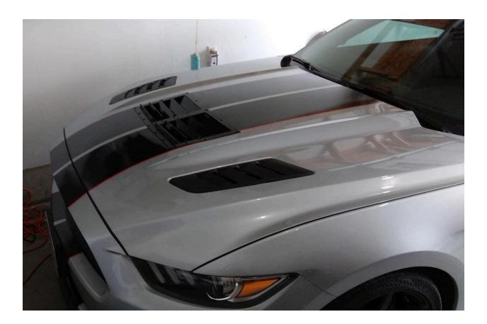
Customer: Bud S. Location: Ontario Vehicle: Mustang Event type: High performance driving events Previous setup: Unknown brand aft mkt side louvers in OE location Extractor setup: Race Louvers single center RT trim 240 sqin with aft mkt side louvers Temperature reductions: 240F to 215F coolant temp reduction
