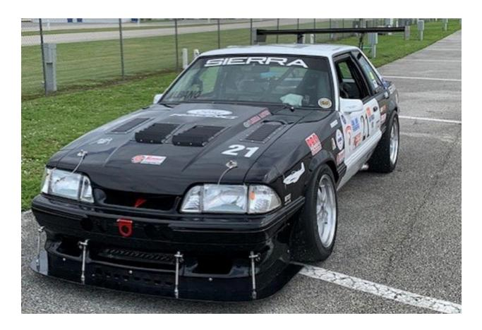
Customer: Michael A. Location: Florida Vehicle: Fox Mustang Event type: Road course racing Previous setup: Unknown brand side stamped louvers only Extractor setup: Race Louvers center RX trim pair 280 sqin with side stamped louvers Temperature reductions: 235F to 200F coolant temp reduction
